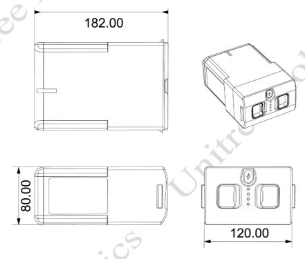
The battery charger is a charging device specifically designed for H1 batteries, with small size, light weight, and convenient portability, providing stable power to the battery.
