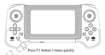
• After modifying the remote control feedback function, it is not saved by default. If you want the changes to take effect the next time you turn on the remote control, hold down the F1 button during shutdown to save the current mode.
