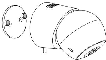
5. Slide the camera onto the mounting plate and make sure it is securely attached.
