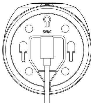
4. For wall mounting, place the cable into the cable channel of the mounting plate.
